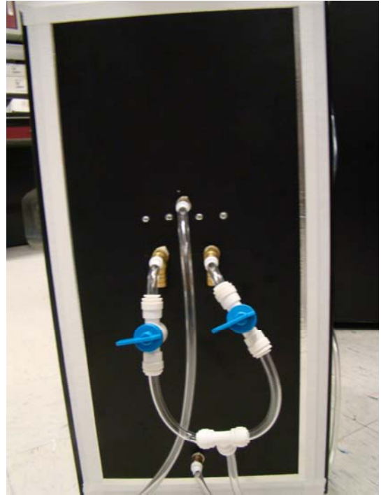
Figure 5. PVC Bypass Valves with "T" Connection
